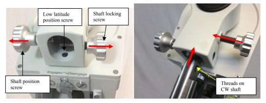
Figure 16. Install the counterweight shaft
